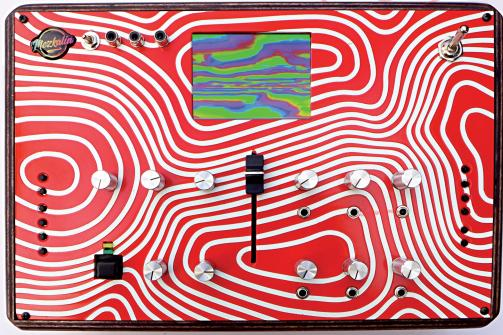
The Landscaper is a no input Feedback Generator, where functions are based on two VGA converter, which creates an INTERNAL FEEDBACK. Each converter has it's own menu to adjust settings.
